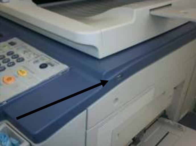
A photograph showing the side of a copier. A black arrow points to a small, dark port on the side panel, which is the flash drive port.                                 |
